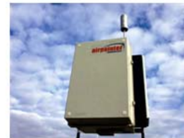
"Compact" Ambient Air Monitoring System (800x600x500mm), Air Monitors, Ltd., USA
